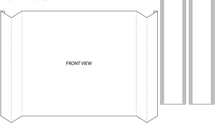
2. Attach back panel covers to rear of display panel as shown, aligning velcro on back panels to velcro on display panel.
